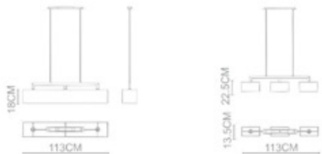
Even 3 Bar Pendant with Big Shade PD-7004 E27 3x40W Polished Chrome+ Stainless Steel Polished
