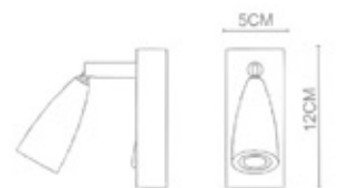
Buzzer Small Arc Wall Lamp WL-50002 LED 1x3W LED Stainless Steel Polished +Polished Chrome
