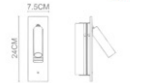
Syphon Round Recessed Wall Lamp+Switch WL-40012 LED 1x3W Stainless Steel Polished+ Polished Chrome 5.7CMx20CM Hole on the wall
