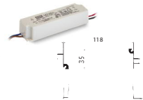
Brand - Meanwell Code - LPC 20-700 Type - Constant Current Watt - 20W IP Rating - IP67 No Of Fixtures - Min 4, Max 8 Dimension:118*35*26mm (L*W*H)
