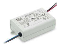
Brand- Meanwell Code- APC-25-700 Type - Constant Current Watt - 25W IP Rating - IP54 No Of Fixtures - Min 1, Max 1 Dimension-84*57*29.5(L*W*H)
